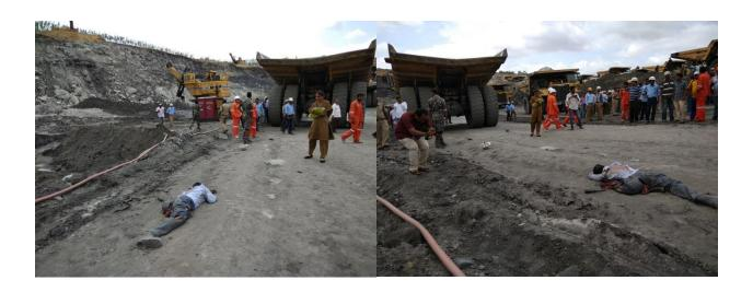
Prima facie cause of the accident: While a supervisor was going on an overburden bench of an opencast coal mine towards a shovel, a 100T dumper, which was going towards the same shovel for taking load, ran over the supervisor, killing him on the spot.
